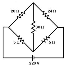
7. Find the voltage to be applied across AB in order to drive a current of 5A [L5,CO1,10M] into the circuit.
