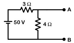
4. Determine the maximum power delivered to the load resistance  $R_L$
