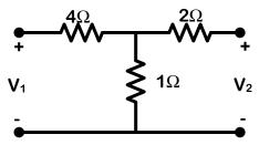
**8.** Find the Short circuit parameters for the given circuit.
